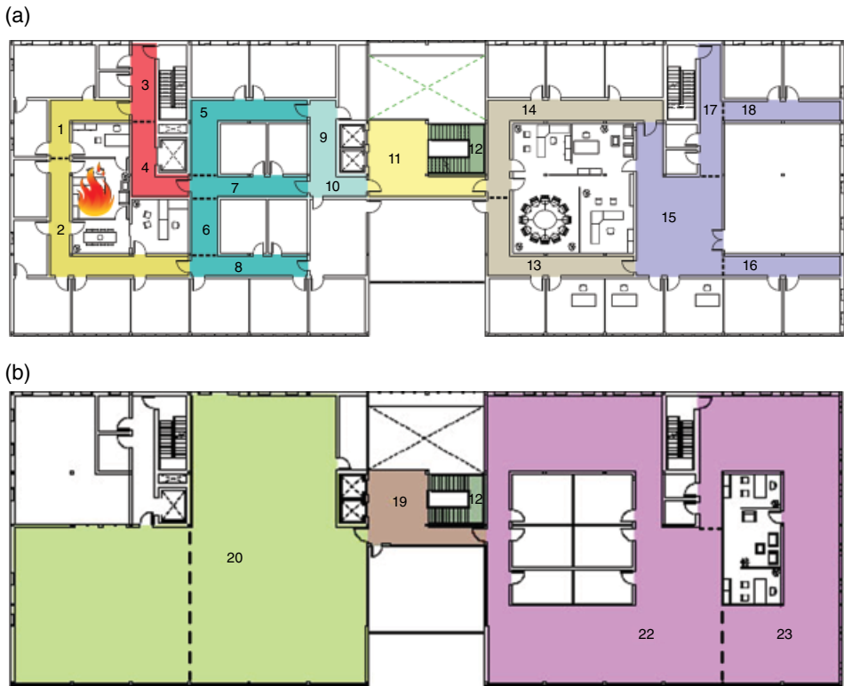
Figure 9.6 (a) Example 9.2: 3 rd Floor smoke zone segments. (b) Example 9.2: 4 th Floor smoke zone segments.
